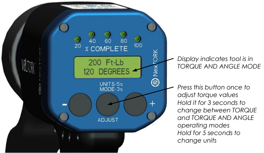
Figure 13 – TOOL DISPLAY IN TURN-OF-THE-NUT MODE
